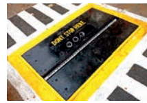
Under Vehicle Scanning System
